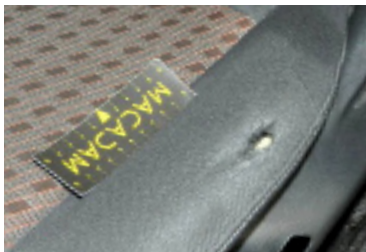
Scheur in de bekleding
